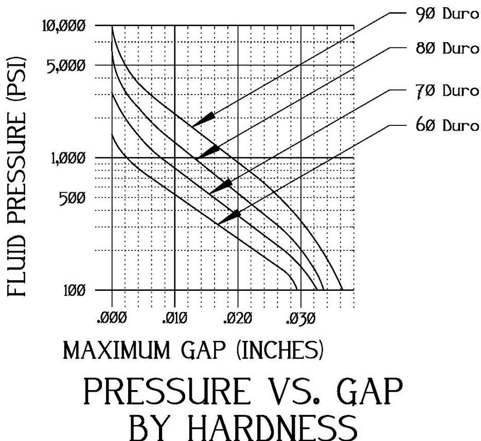
The hardness of the o-ring compound determines the radial gap that may be sealed at any given operating pressure. The harder the compound, the higher the pressure and/or the wider the gap that may be handled by the design. Hardness of most o-ring compounds is
