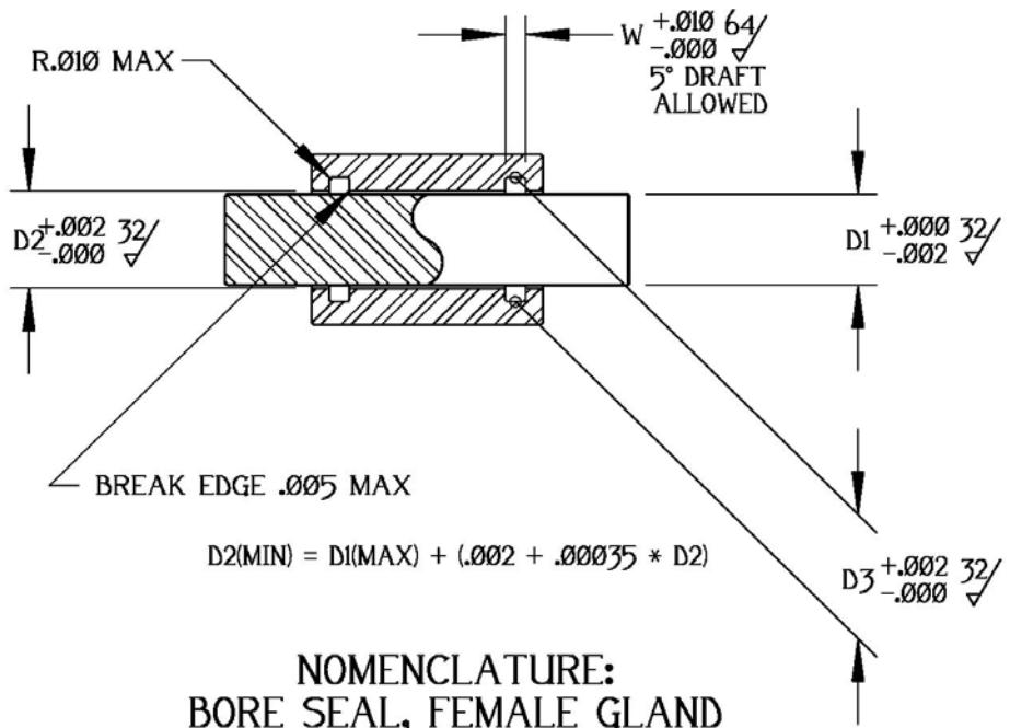
Gland geometry for this kind of seal is controlled by SAE ARP-1232 (Static) or SAE ARP-1233 (Dynamic).
